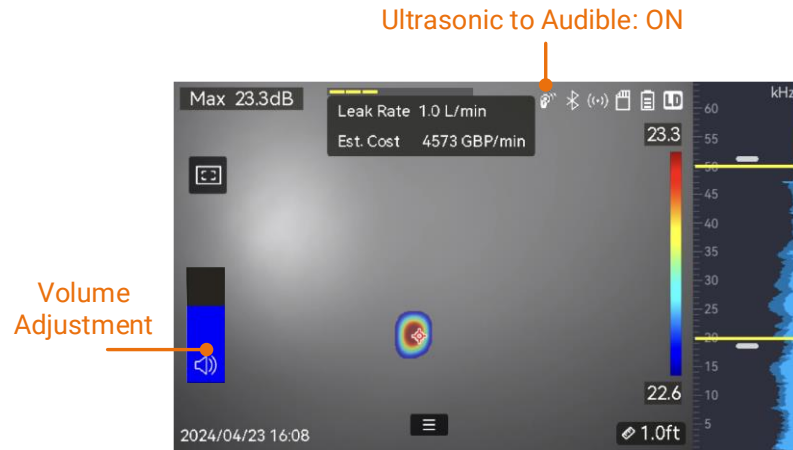
Figure 5-4 Ultrasonic to Audible and Volume Adjustment
