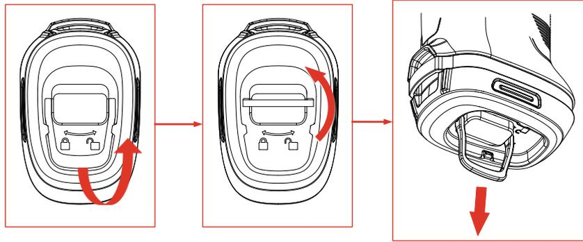
Figure 3-1 Removing Battery
