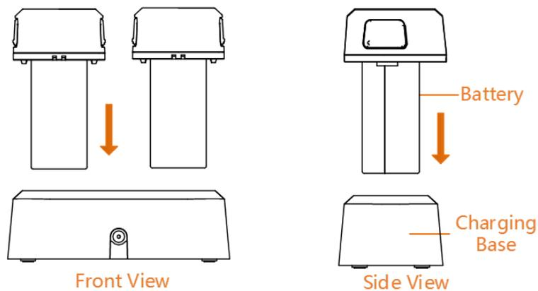
**Figure 2-2 Charge Battery**
