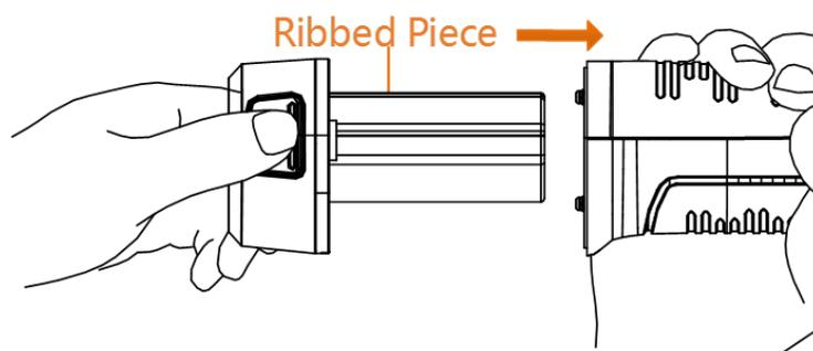
**Figure 2-3 Insert Battery**
